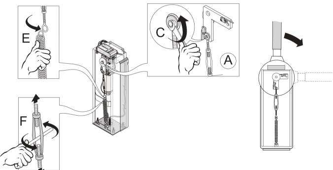
STEP 9 With the spring unloaded, hook upper part of tie to support (A) and screw bolt (C) with an adjustable spanner. After this operation, hook the spring to the rod.
