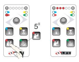
Press for 5 seconds, the red LED **(SX)** will light and then switch off.
