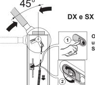
Open door (1) insert key(2) & unlock with 3 clock-wise rotations. See scheme.
